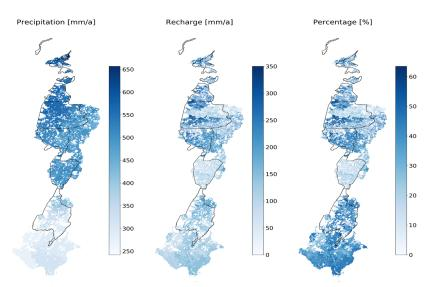
Figure 1: Annual means of precipitation, recharge, and the recharge/precipitation ratio on HRU level for 1990-2018
