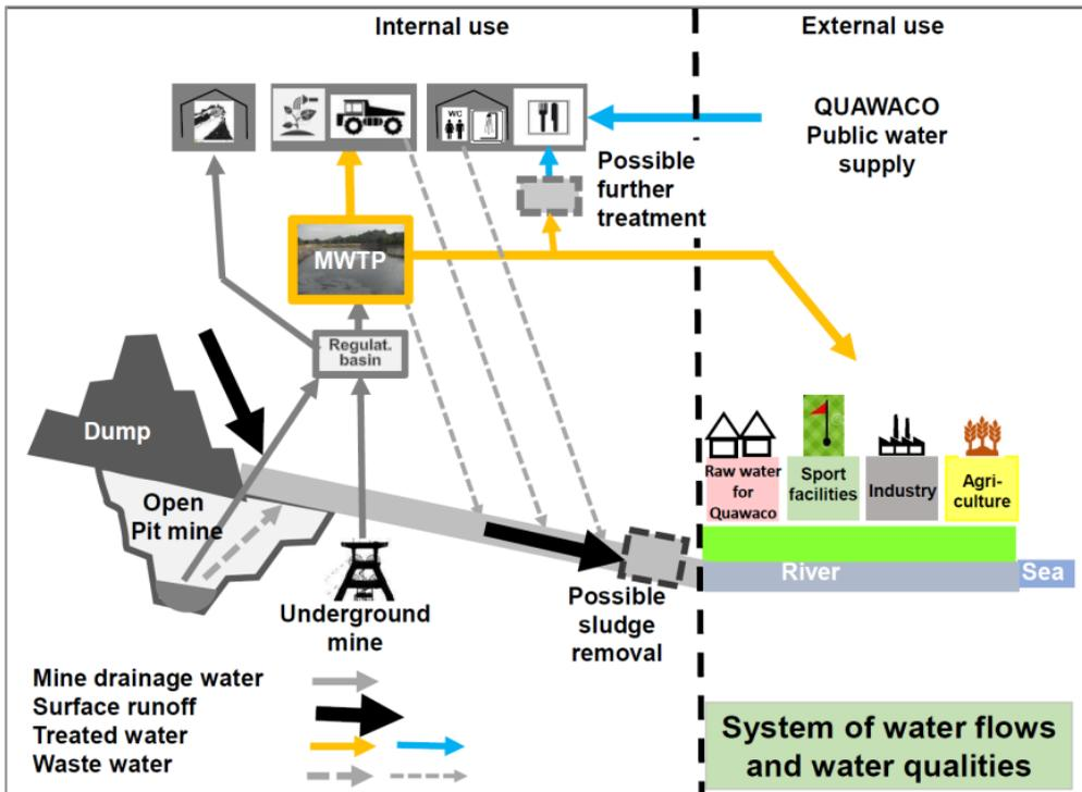
Figure 3 Elements of the mine water system in Hon Gai (eE+E)
